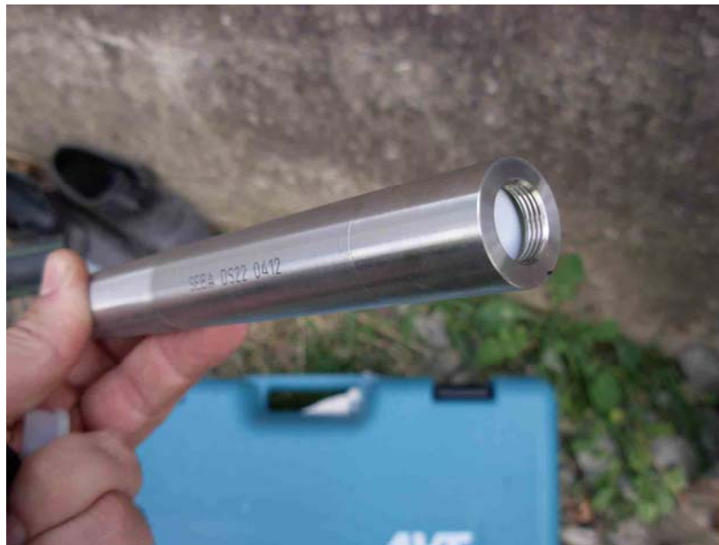
Sonde for measuring H (cm) & T (°C)
