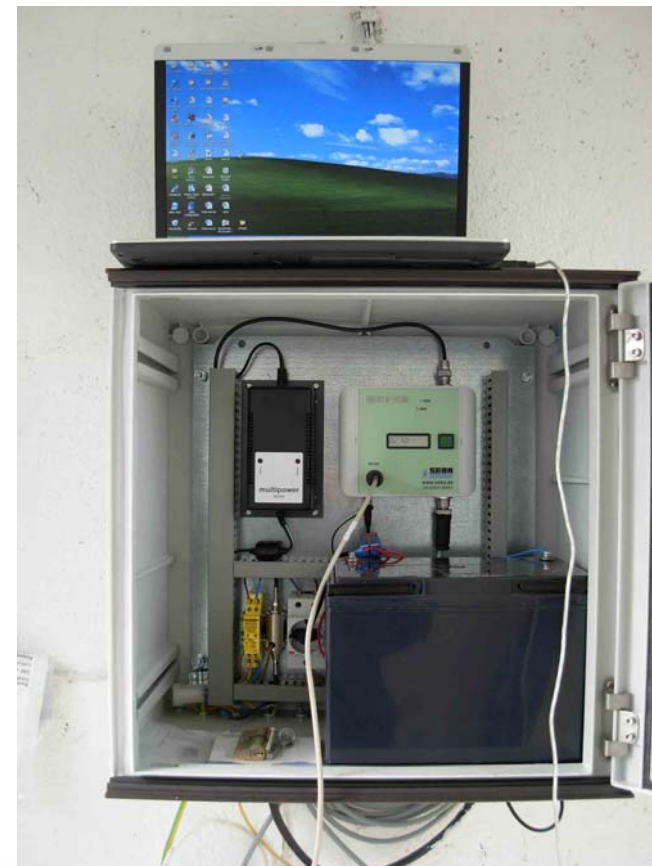
Data Logger MDS-5 for collecting data with GSM/GPRS modem for transmitting data
