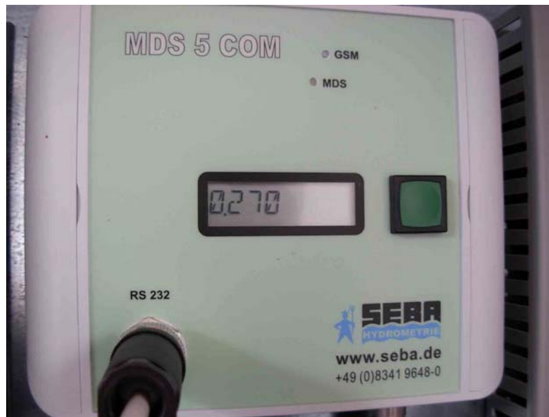
Data Logger MDS-5 for collecting data with GSM/GPRS modem for transmitting data
